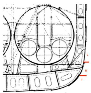
Left: An extract from а midsection plan of *Olympic* and Titanic, showing a cutaway view of the ship at boiler room 2. The letters in red mark the locations of the strakes of hull plating, J, K and L. The thick red lines mark the approximate location of the rivetted landings between (top) strakes L and K and (bottom) strakes K and J. (The Shipbuilder, 1911/Ioannis Georgiou collection)
